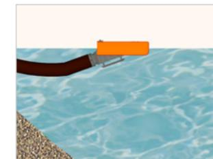
**DEEP DRAFT** – Strainer drafts from a few inches below surface where water is cleanest. Note how hose weight tilts strainer position while float remains level. *Right photo*
