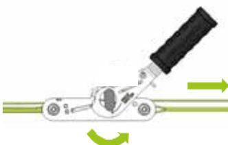
Pull the strap release knob and guide the strap through the strap guide, to elongate the strap.
