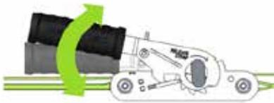
Hold the handle and push down until the control pin slides in the control slot (1). Then pull up (2).
