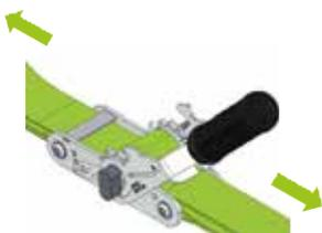
Hold the strap at both ends and pull them simultaneously.
