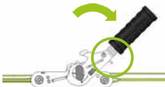
Pull the operation lever and set the handle to full release position.
