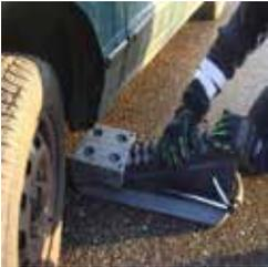
Place the stair under the object to be stabilized.
