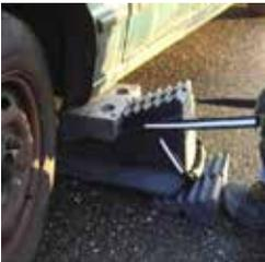
When a little more pressure is required, it's possible to push a wedge underneath the Rapid Stair.
