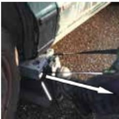
Keep on pulling the strap while the load is going up.
