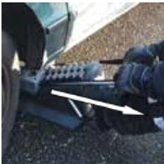
Pull the strap of the Saddle Wedge firmly until it's stuck between the stair and the object.
