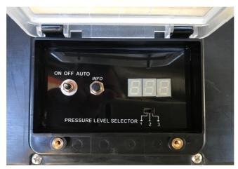
In "AUTO" mode electronic board restores automatically the level of the operative pressure of the pneumatic arches in case of a pressure decreasing due to a big thermal excursion or a light damage on the supporting structure.
